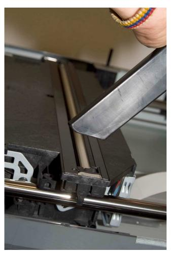
Hold the nozzle above the light and over the gap in the scanning head. Move it from side to side to side being careful not to touch the tube.
