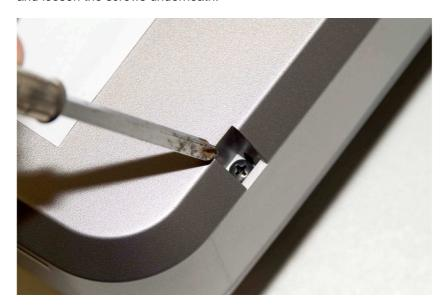
On the back of the machine you will find one other screw to be removed completely.
